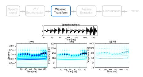
CWT: continuous wavelet transform BWT: bionic wavelet transform SSWT: synchro-squeezed wavelet transform
